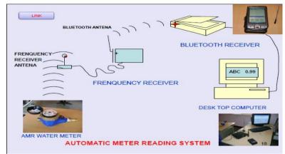
Fig.2 Automatic meter reading system
