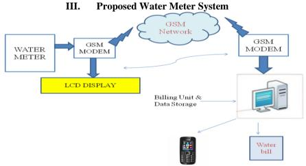
Fig.3 Proposed system block diagram
