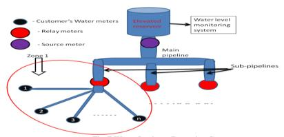
Fig.7 Water Leakage Detection System
