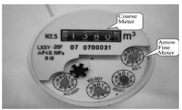
Fig.1 Mechanical Water Meter
